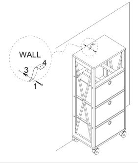
\*\* WE RECOMMEND THAT YOU PERIODICALLY TIGHTEN ALL BOLTS AND SCREWS WITH PHILLIPS HEAD SCREWDRIVER, NOT INCLUDED.
