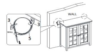
\*\* WE RECOMMEND THAT YOU PERIODICALLY TIGHTEN ALL SCREWS USING PHILLIPS HEAD SCREWDRIVER, NOT INCLUDED.
