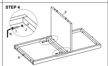
A. ATTACH DIVIDER (F) TO TOP (A) WITH BOLTS (I), FLAT WASHERS (J) AND LOOSELY TIGHTEN USING ALLEN WRENCH (K).
