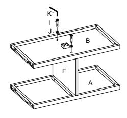
A. ATTACH SHELF (B) TO DIVIDER (F) WITH BOLTS (I), FLAT WASHERS (J) AND LOOSELY TIGHTEN USING ALLEN WRENCH (K).
