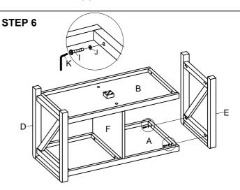
A. CONNECT RIGHT SIDE FRAME (D) TO TOP (A) AND SHELF (B) WITH BOLTS (I), FLAT WASHERS (J) AND LOOSELY TIGHTEN USING ALLEN WRENCH (K).
