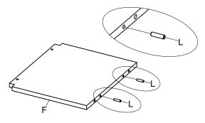
A. INSERT WOOD DOWELS (L) INTO DOWEL HOLES ON DIVIDER (F).
