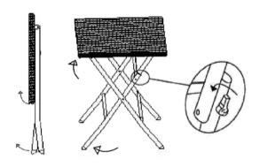
A. TO CLOSE - TURN THE LATCH MECHANISM TO UNLOCK TABLE TOP.
