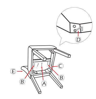
Partly screw in bolts, but do not fully tighten
